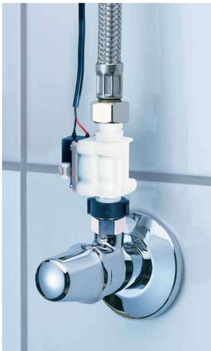
Solenoid valve mounted under wash basin, directly onto angle valve
