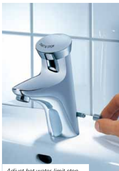
Adjust hot water limit stop
