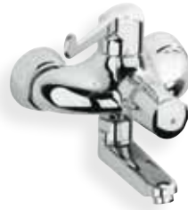
34 019 000 Grotherm Ergomix Thermostatic basin mixer, 1/2", lever for elbow operation, metal elbow lever 170 mm, temperature handle with safety stop, easy thermal disinfection, projection 178 mm
