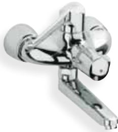
34 020 000 Grotherm Ergomix Thermostatic basin mixer, 1/2", lever for elbow operation, metal elbow lever 250 mm, temperature handle with safety stop, easy thermal disinfection, projection 255 mm, covered S-unions
