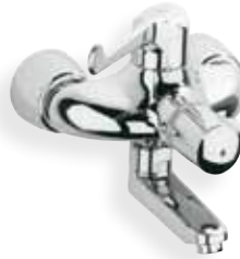
34 021 000 Grotherm Ergomix Thermostatic basin mixer, 1/2", lever for elbow operation, metal elbow lever 170 mm, temperature handle with safety stop, easy thermal disinfection, projection 195 mm, covered S-unions
